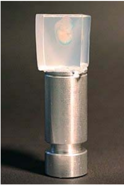
Fig. A1f Agarose Block Attached to Mount
